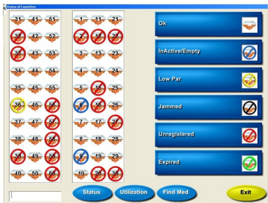
The KL60 shows full cassette information of all 60 cassettes, including empty cassettes, empty slots, par level, etc.
