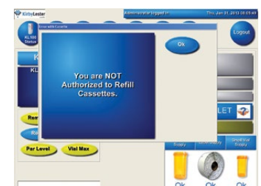
FillSafe™ security system prevents dispensing from a cassette that was not authorized by an RPh.
